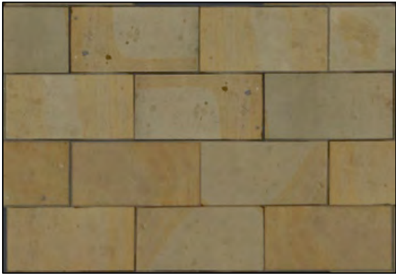
Footpaths: Charcon Stonemaster 450x300x80mm mix of 3 colours: 60% medium; 30% light; 10% dark
